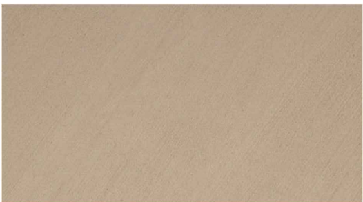
P2 Waterfront edge: insitu concrete/ coloured concrete Solutions (CCS) : Colour/Size: paperbark coloured full body oxide colour 20mm river gravel Finish: honed
