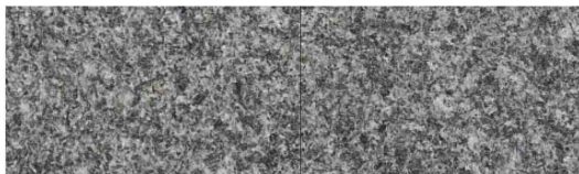
Long bands- in Tier 1 and 2 Material: raven black/ gray granite unit paver Size: 600x300x40mm Finish: exfoliated finish Pattern: long band
