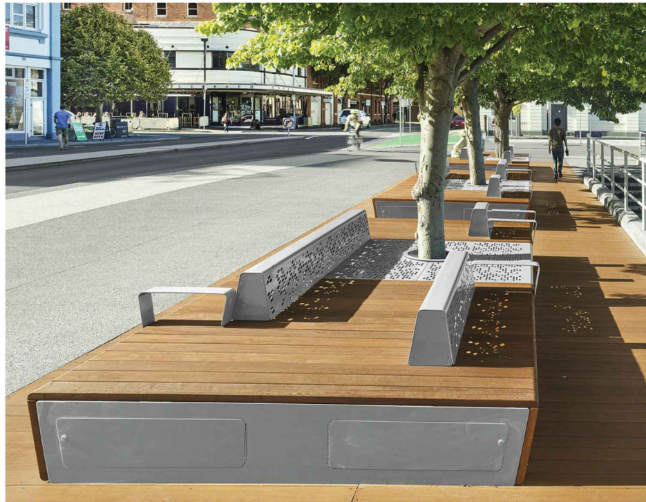
feature seating within promenade: seasoned hardwood timber and perforated metal: alignment will be adjusted as per actual location
