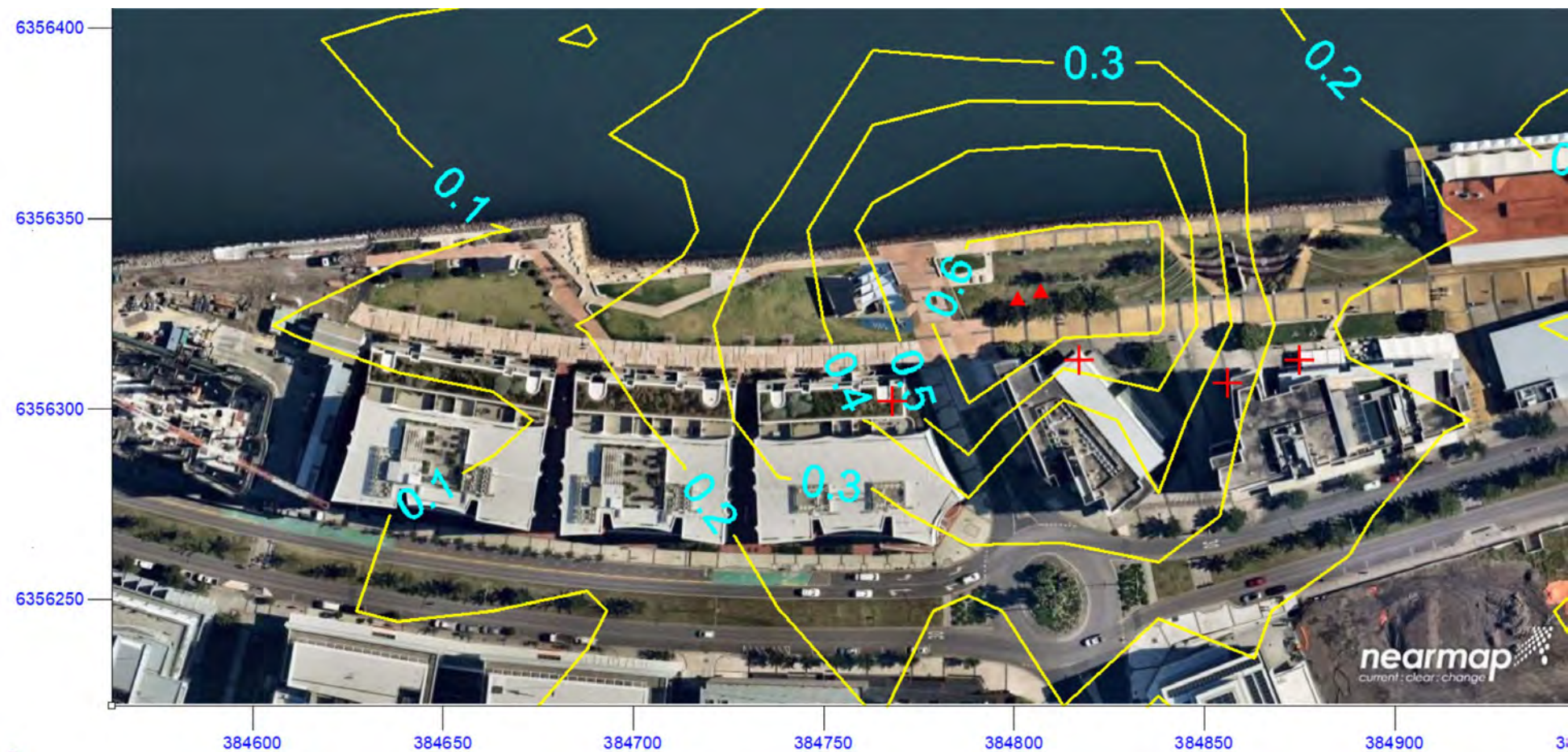
Figure 4 Predicted odour concentration contours at the ground level (hourly 100 th percentile)
