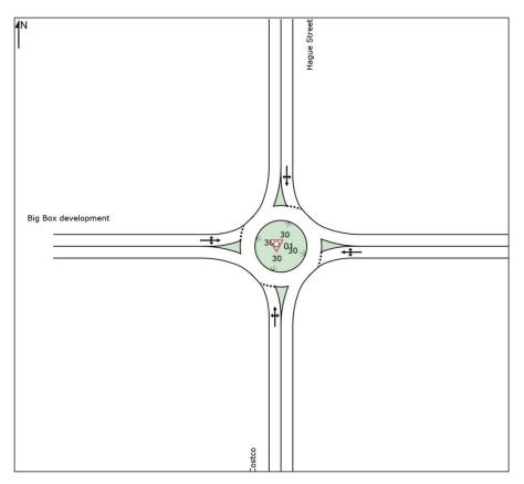
Figure 5-3 Proposed internal roundabout layout at southern end of Hague Street
