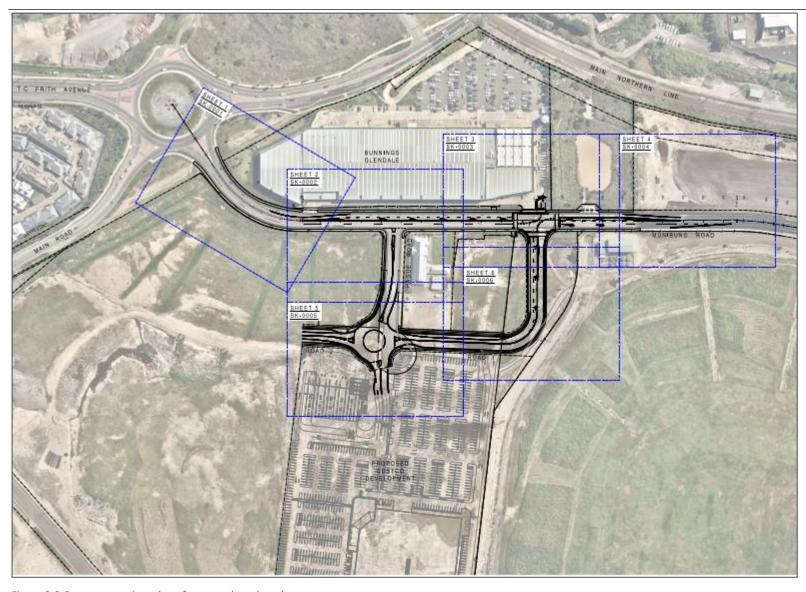
Figure 3-2 Concept overview plan of proposed road works
