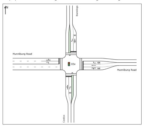
Figure 5-1 Proposed signalised intersection layout of Munibung Road/Bunnings Access/Costco Access
