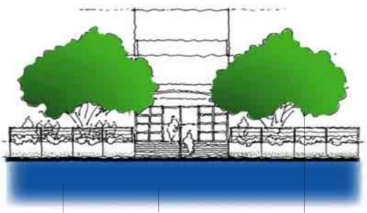
Foreshore Terrace Walling including insitu concrete panels and balustrade sections aligning with pavement panels, tidal line sand blasted into lower section of wall.
