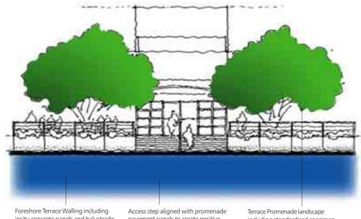
Foreshore Terrace Walling including insitu concrete panels and balustrade sections aligning with pavement panels, tidal line sand blasted into lower section of wall.
