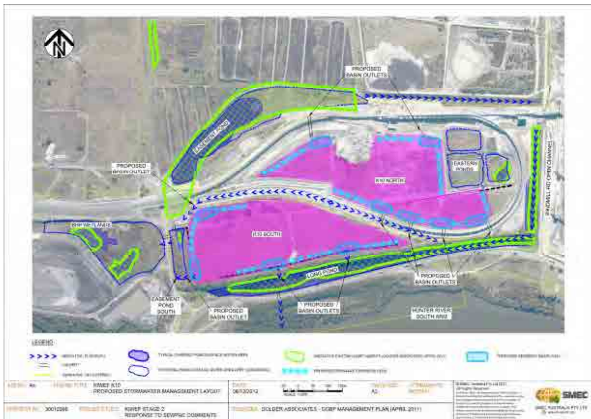
Plate 5: Figure 4a – K10 Capping Area showing GGBF Habitat Areas and Proposed Stormwater Management Controls
