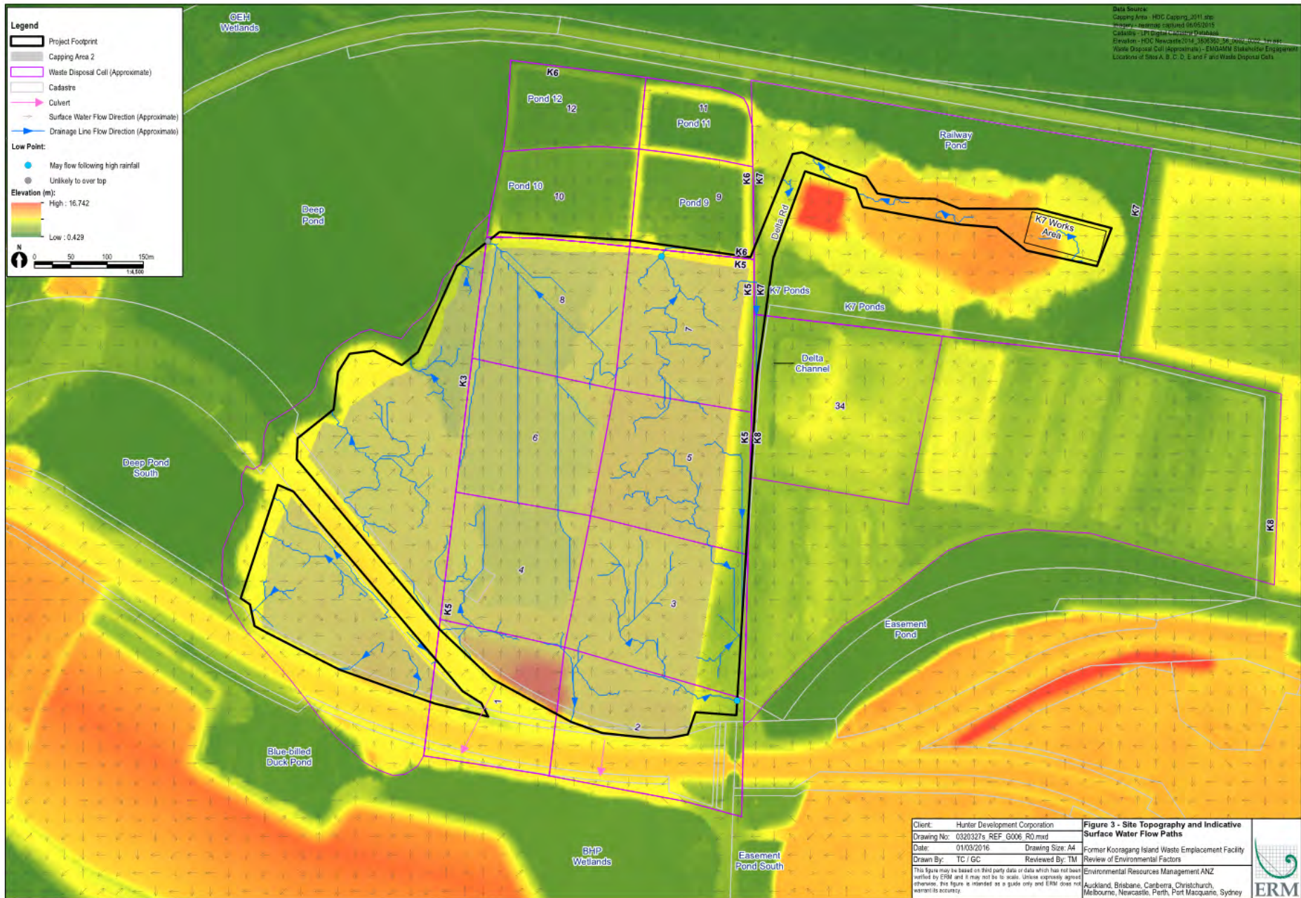
Figure 2 – Area 2 - Topography and Indicative Surface Water Flow Paths – Existing Conditions (source: ERM 2016)
