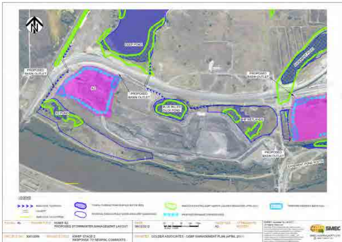
Plate 2: Figure 4B – K2 Capping Area showing GGBF Habitat Areas and Proposed Stormwater Management Controls
