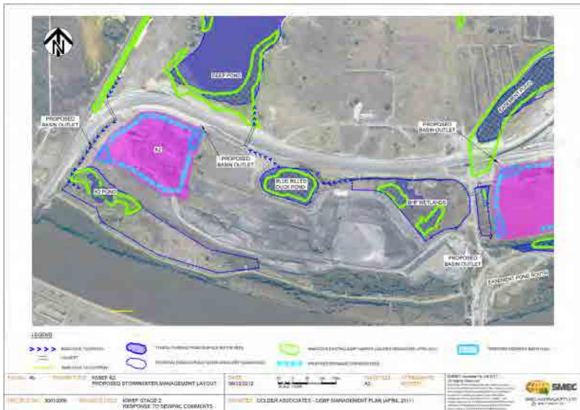
Plate 6: Figure 4B – K2 Capping Area showing GGBF Habitat Areas and Proposed Stormwater Management Controls
