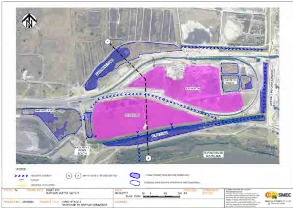
Plate 19: Figure 1b – Surface Water Layout at KIWEF BPond Areas and Overflow Paths
