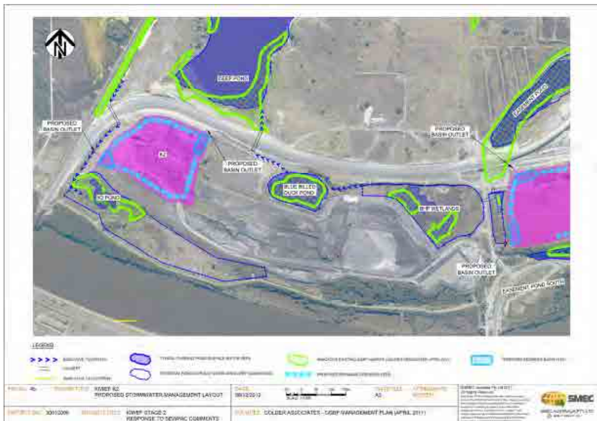
Plate 15: Figure 4B – K2 Capping Area showing GGBF Habitat Areas and Proposed Stormwater Management Controls
